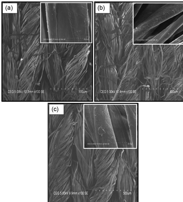
Fig. 3 — SEM of (a) control, (b) cationised samples and (c) enzyme treated cationised samples (500 µm) (inset 20µm)
