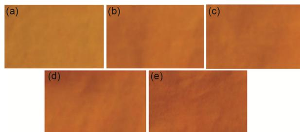
Fig. 1 — Visual observation of dyed sample (a) conventionally dyed, (b) cationised dye, (c) ultrasonicated cationised dyed, (d) enzyme treated and cationised dyed and (e) ultrasonicated enzyme and cationised (combined) dyed
