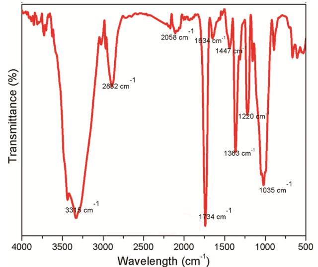
Fig. 4 — FTIR of cationised cotton sample
