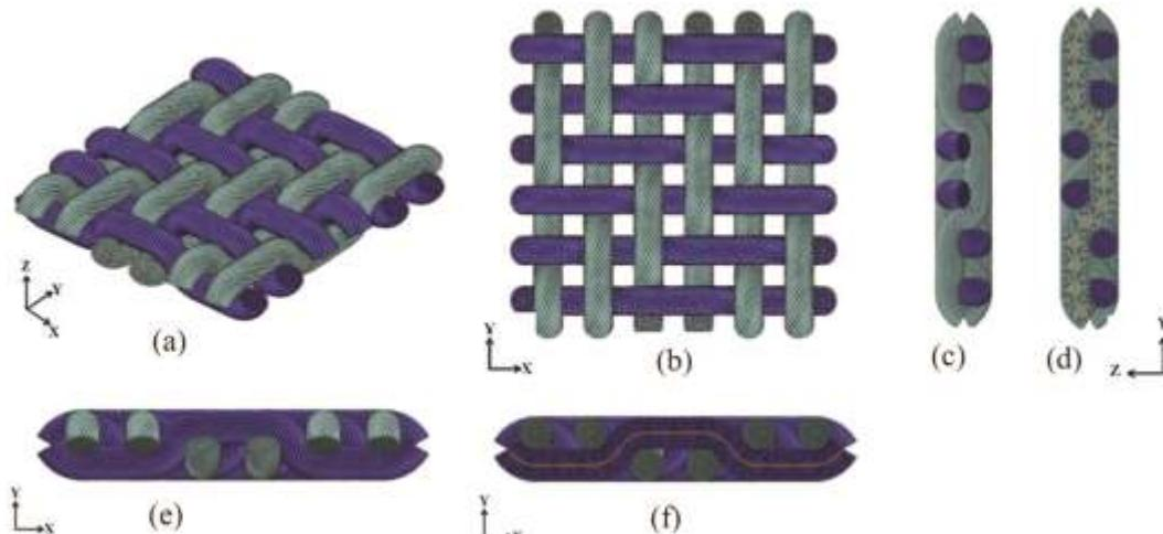
Fig. 5 — CAD of 2x2 twill weave fabrics(a) isometric view, (b) top view, (c) side view, (d) cross-section at center line of yarn path for weft yarn, (e) front view, and (f) cross-section at center line of yarn path for warp yarn<sup>13</sup>
