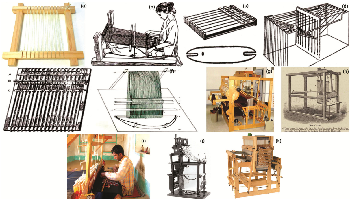
Fig. 5 — (a) Wooden frame with warp 66 , (b) body loom (“Shed Stick” method) 65 , (c) Home-made frame loom and shuttle 65 , (d) Box Loom (with rigid heddle lowered) 65 , (e) Home-made Frame Loom 65 , (f) loin loom 67 , (g) cottage loom 68 , (h) fly shuttle loom 69 , (i) pit loom 70 , (j) Jacquard loom 71 and (k) dobby loom 72
