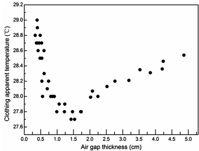
Fig. 4—Scatter plot of clothing surface temperature and air gap thickness
