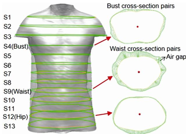
Fig. 1—Cross-section pairs on garment B96
