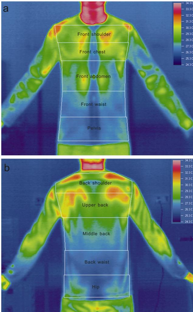
Fig. 2—Ten temperature measuring zones (a) frontal body, and (b) rear body
