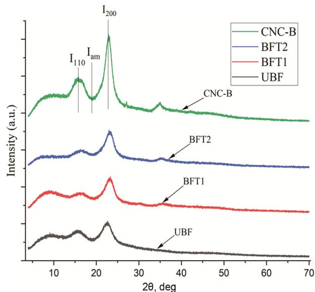
Fig. 5 — XRD results of banana fibres and cellulose nano-crystal
