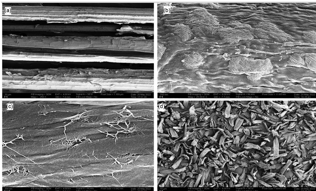
Fig. 4 — FESEM images of banana fibres (a) untreated, (b) alkali-treated, (c) bleached and (d) nano-crystal
