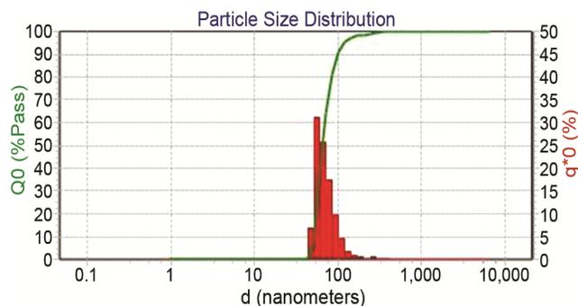
Fig. 2 — DLS analysis of banana cellulose nano-crystal
