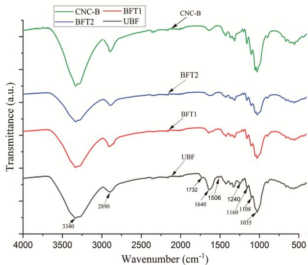
Fig. 6 — FTIR spectra of banana fibres and cellulose nano-crystal
