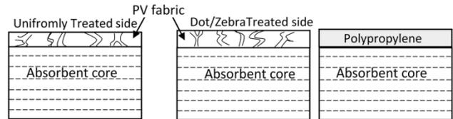
Fig. 4 — Different configuration of the rewet test
