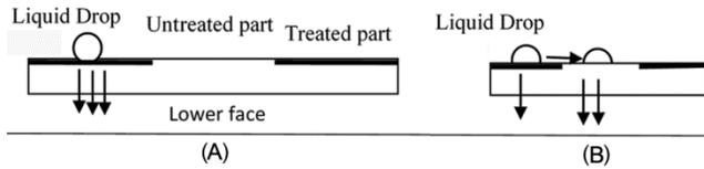
Fig. 6 — Fluid movement across the PV fabric (A) 1 cm stripe width and (B) 0.5 cm stripe width
