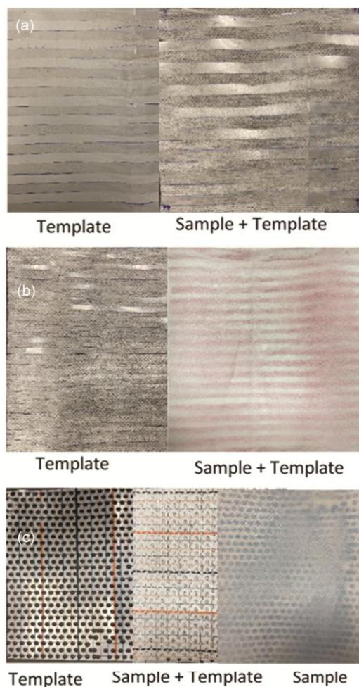
Fig. 2 — Spray pattern/template with stripe width (a) 1 cm, (b) 0.5 cm and (c) dot pattern
