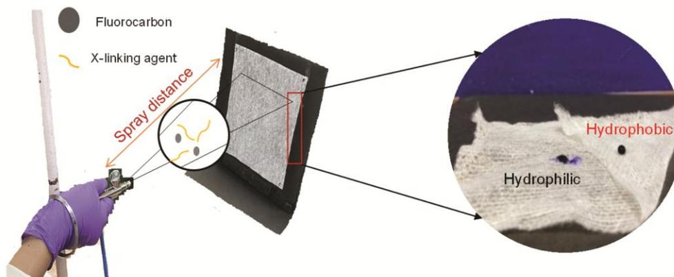
Fig. 1 — Spray coat technique
