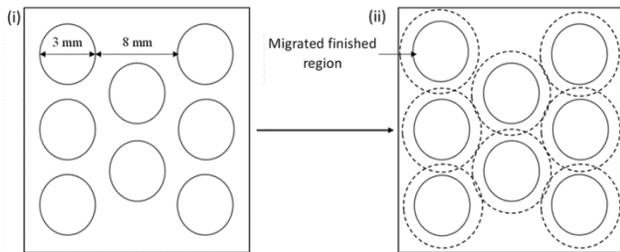
Fig. 7 — Schematic representation of dot pattern (i) before and (ii) after application of finish
