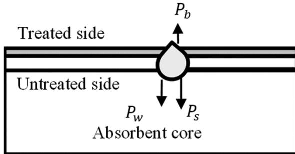
Fig. 10 — Ejection of liquid droplet through uniformly treated PV fabric
