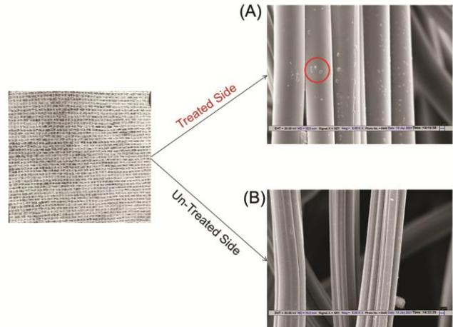
Fig. 5 — SEM image analysis (A) coating (front) side and (B) back side of polyester-viscose spun-lace nonwoven fabric
