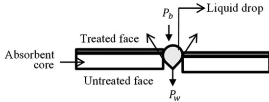
Fig. 9 — Penetration of liquid droplet through PV fabric
