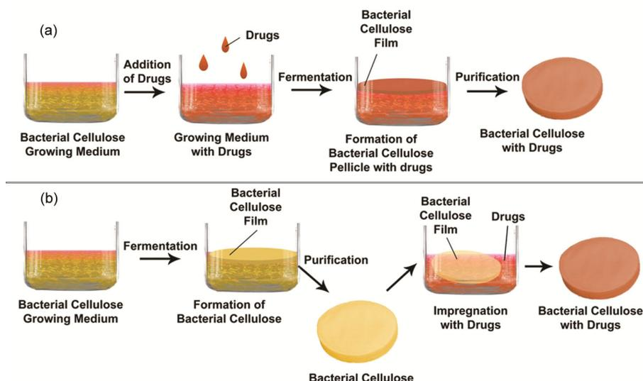
Fig. 4 — Schematic illustration of bacterial cellulose based composite wound dressing development by (a) *in-situ* method and by (b) *ex-situ* method
