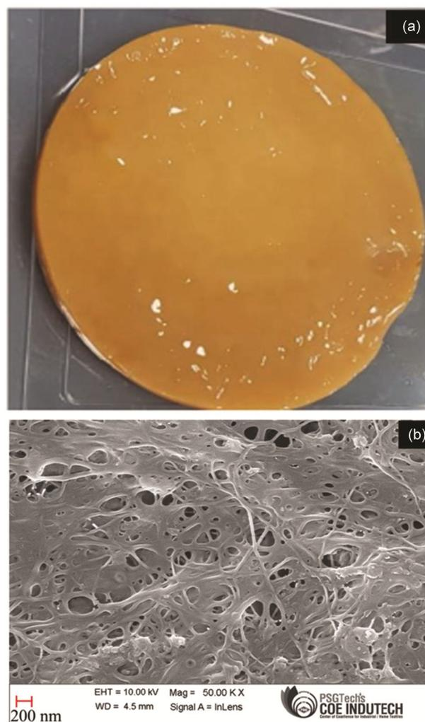
Fig. 2 — (a) Physical appearance of fermented bacterial cellulose after 20 days without purification, and (b) SEM image of three-dimensional fibre network structure
