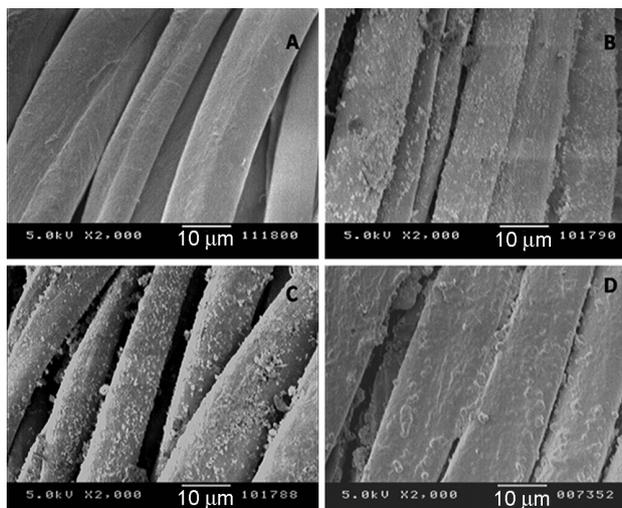
Fig. 3—SEM images of (A) control cotton, (B)  $\text{TiO}_2/\text{SiO}_2$  without plasma, (C)  $\text{TiO}_2/\text{SiO}_2$  with plasma, and (D)  $\text{TiO}_2/\text{SiO}_2$  with plasma and polymer deposition
