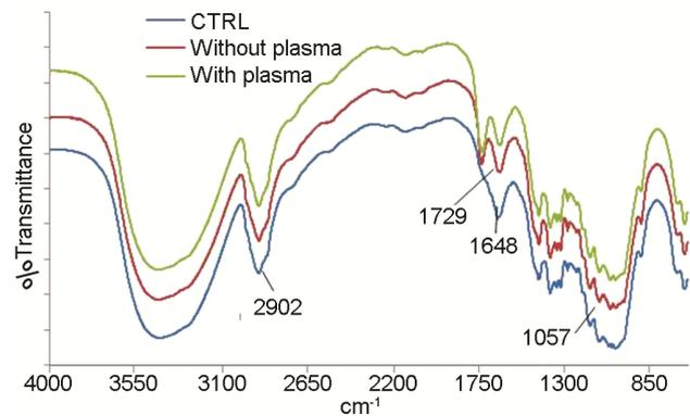
Fig. 5—FTIR spectra of BTCA treated samples, control cotton, without plasma and plasma
