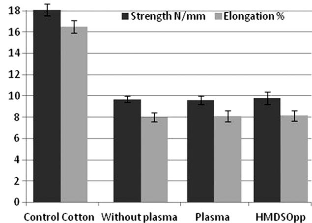
Fig. 6—Tensile strength and elongation of finished samples
