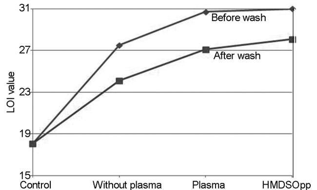
Fig. 2—Effect of washing on LOI values of the finished samples
