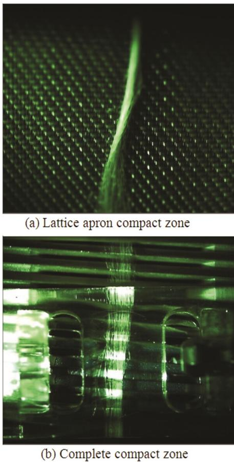
Fig. 5 — Fibre sliver in compact zone
