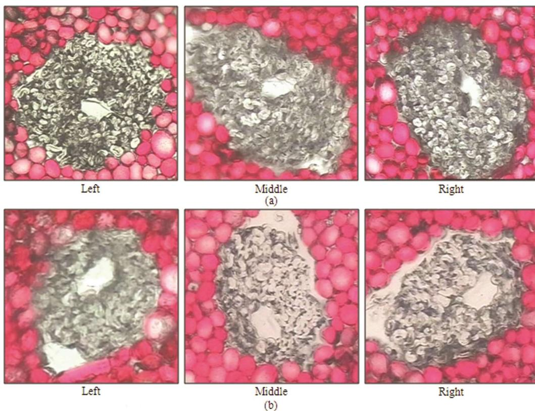
Fig. 4 — Cross-section of (a) 29.2tex /44.4dtex and (b) 14.6tex/44.4dtex complete condensed siro-spinning core-spun yarns
