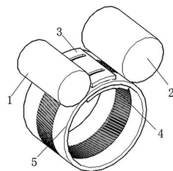
Fig. 1 — Structure of CCSS [1-Output top roller, 2-Front top roller, 3-Airflow guiding device, 4-Air suction card, and 5- Perforated hollow roller]
