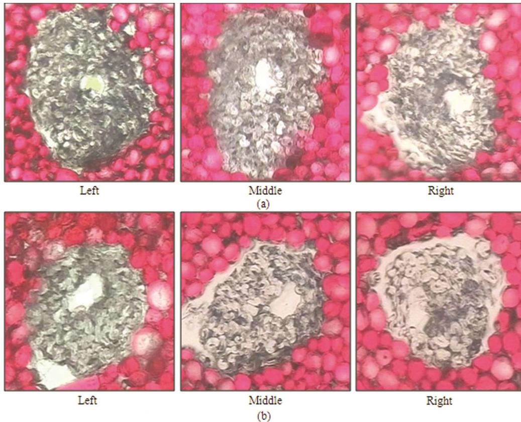
Fig. 3 — Cross-sections of (a) 29.2tex /44.4dtex and (b) 14.6tex/44.4dtex lattice apron compact siro-spinning core-spun yarns
