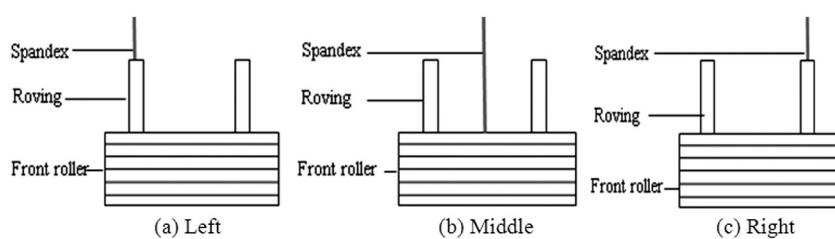
Fig. 2 — Different feed positions of core filament
