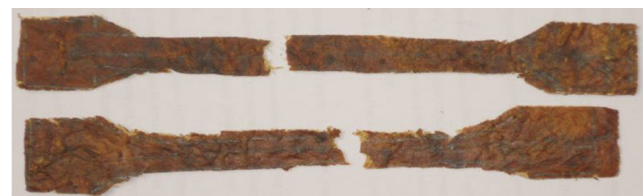
Fig. 1 — Ruptured composite samples after tensile testing
