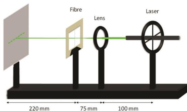
Fig. 1—Experimental set-up for diffraction pattern detection of textile fibres
