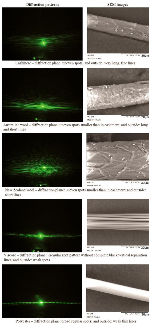
Fig. 2—Diffraction patterns and corresponding SEM pictures of different textile fibres
