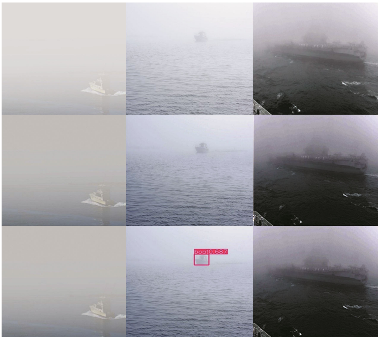
Fig. 5 — Detection effect of dehaze enhancement method based on AOD network
