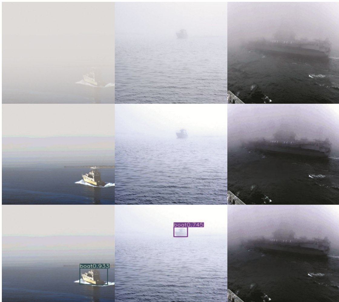
Fig. 4 — Detection results of dark channel prior based dehaze enhancement method
