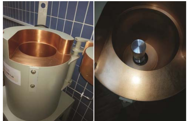
Fig. 2 — Top view of the HPGe detector and shielding system.
