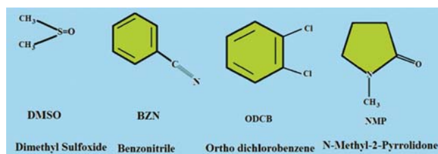
Fig. 15 — Molecular structures of common organic solvents used for graphene liquid phase exfoliation.
