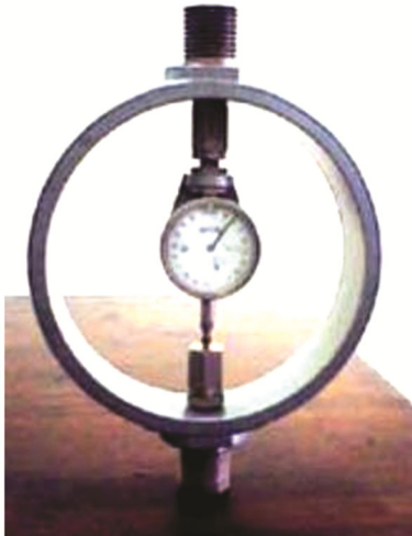
Fig. 1 — A dial gauged force transducer (or, force proving instrument) 2 .
