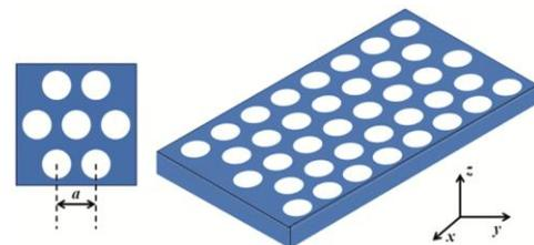
Fig. 2 – Triangular lattice formed by air columns in LiNbO<sub>3</sub> slab.
