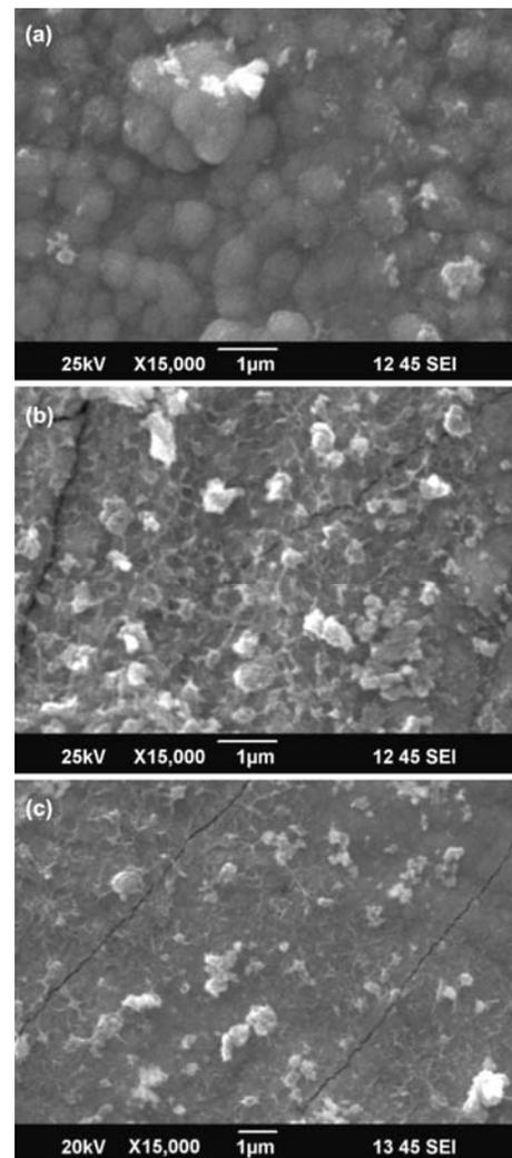
Fig. 2 — SEM images of Fe-W electrodeposited thin films for 45 min at (a)  $20 \text{ mA cm}^{-2}$  (b)  $25 \text{ mA cm}^{-2}$  (c)  $30 \text{ mA cm}^{-2}$
