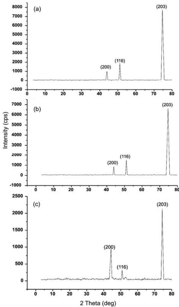
Fig. 1 — XRD images of Fe-W electrodeposited thin films for 45 min at (a)  $20 \text{ mA cm}^{-2}$  (b)  $25 \text{ mA cm}^{-2}$  (c)  $30 \text{ mA cm}^{-2}$
