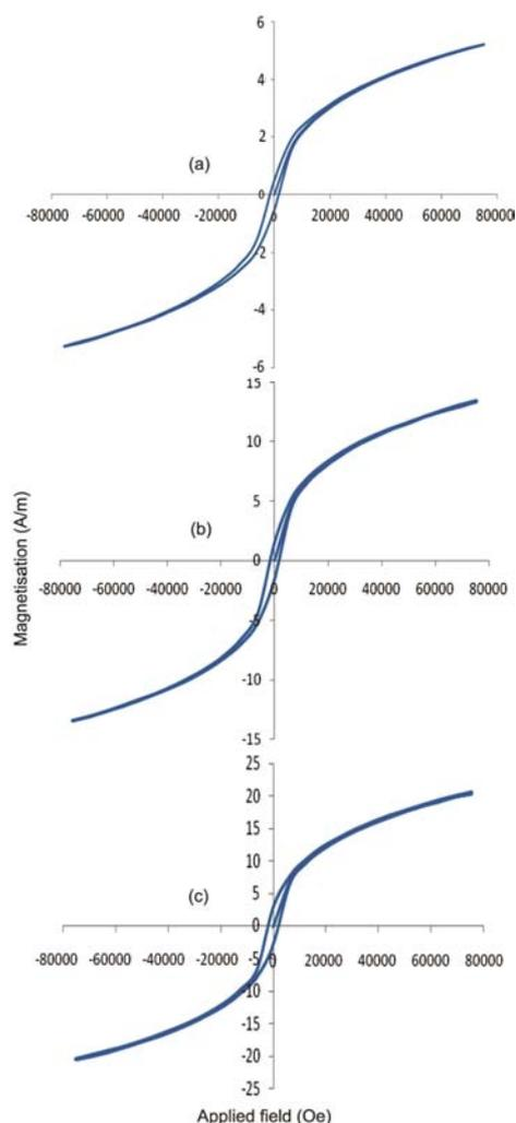
Fig. 3 — VSM images of Fe-W electrodeposited thin films for 45 min at (a)  $20 \text{ mA cm}^{-2}$  (b)  $25 \text{ mA cm}^{-2}$  (c)  $30 \text{ mA cm}^{-2}$
