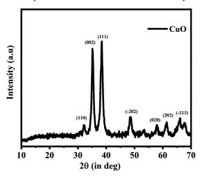
Fig. 1 — XRD pattern of copper oxide
