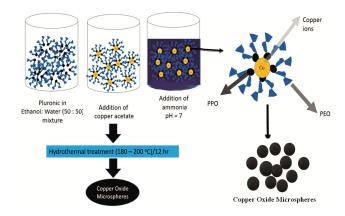
Fig. 3 — Schematic diagram for formation of micelles
