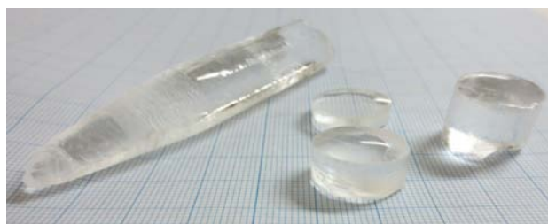
Fig. 1 — Grown TGS-NiSO 4 crystal by SR Method after cutting
