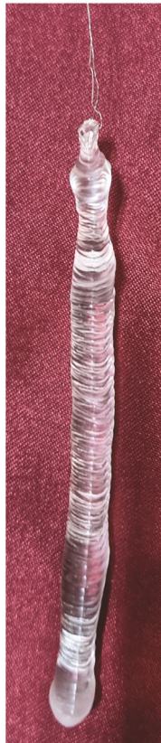
Fig. 5 — A photograph of a potassium chloride crystal grown on the newly developed system
