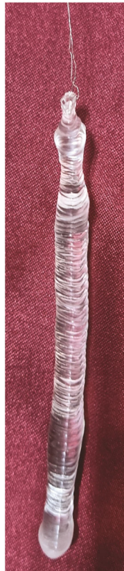
Fig. 5 — A photograph of a potassium chloride crystal grown on the newly developed system
