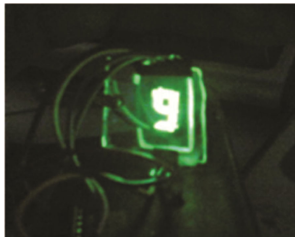
Fig. 5 — Photograph of the green emitting seven segment display prepared in the same device design as that of the green PhOLED reported here. The seven segment display was connected to a digital counter circuit and the photograph was captured at the digital count of 9.
