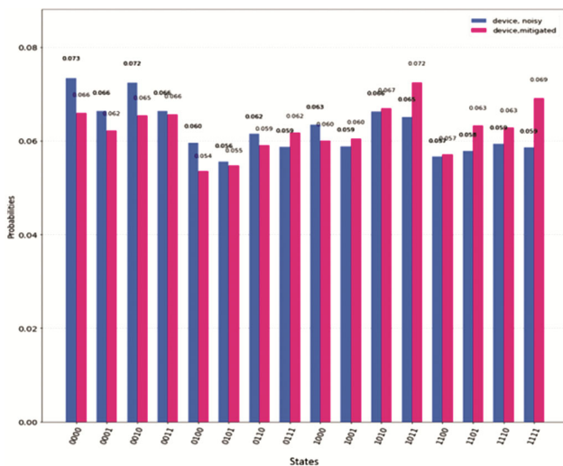
Fig. 6 — Accuracy of 3-qubit implementation of Grover’s algorithm for searching |1111\rangle state with measurement errors and mitigated measurement errors.
