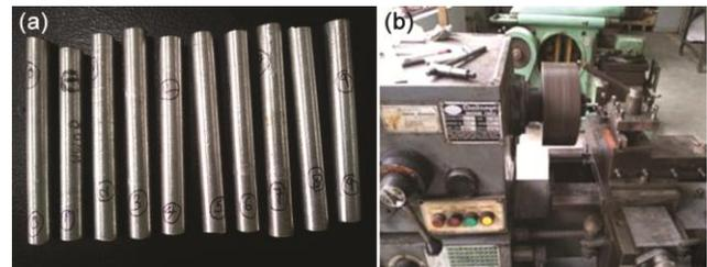
Fig. 3 — (a) Specimens for machinability study (b) Lathe machine for machinability study
