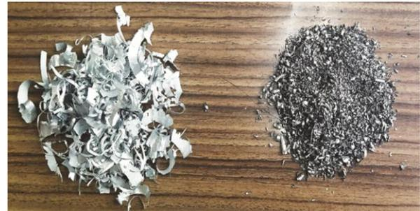
Fig. 5 — Chips formed during machining of as-cast Al 7075 and composite specimen
