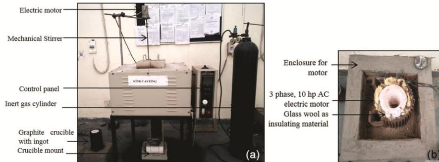
Fig. 2 — (a) Conventional mechanical stir casting setup (b) electromagnetic stirrer
