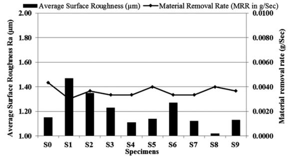
Fig. 4 — Material removal rate and surface roughness of specimens
