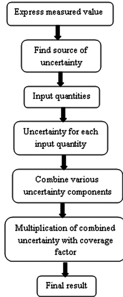
Fig. 1 — Steps to calculate uncertainty of measurement using LPU/ GUM<sup>9-12</sup>
