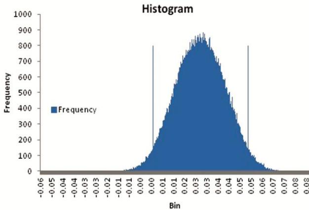
Fig. 3 — A Gaussian shaped histogram from MCS with low and high point.
