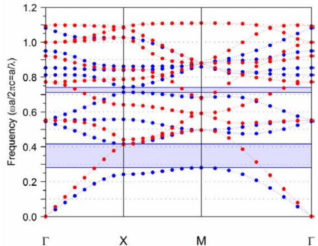
Fig. 2 — Band structure of the basic PhC
