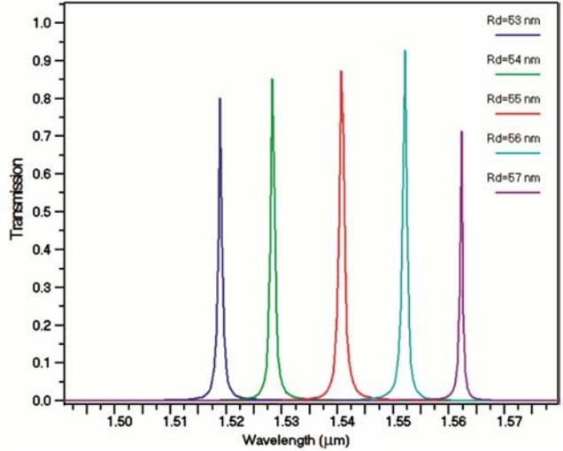
Fig. 5 — Output spectra of the filter for different values of  $R_d$
