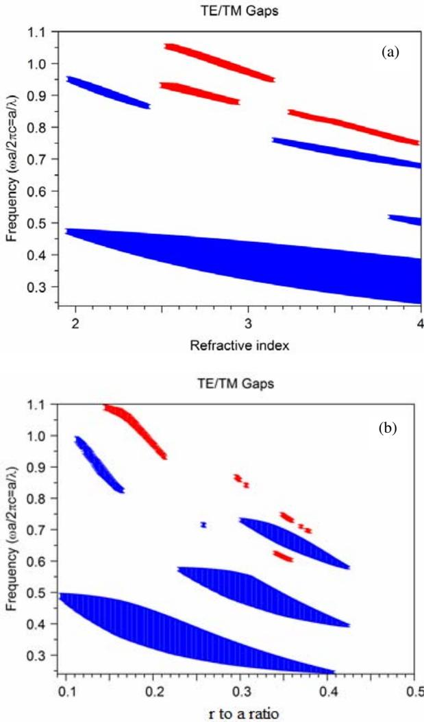
Fig. 1 — Variation of PBG region versus (a) refractive index and (b) radius to period ratio
