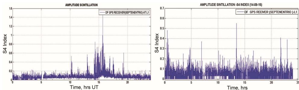
Fig. 5 —  $S_4$  index from Septentrio- dual frequency receiver at L1 band at Delhi
