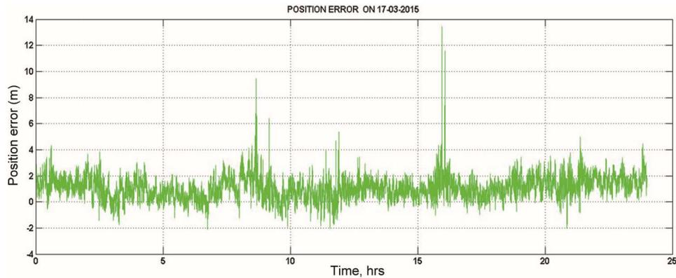
Fig. 6 — Position error measured in the hybrid mode on 17 March 2015
