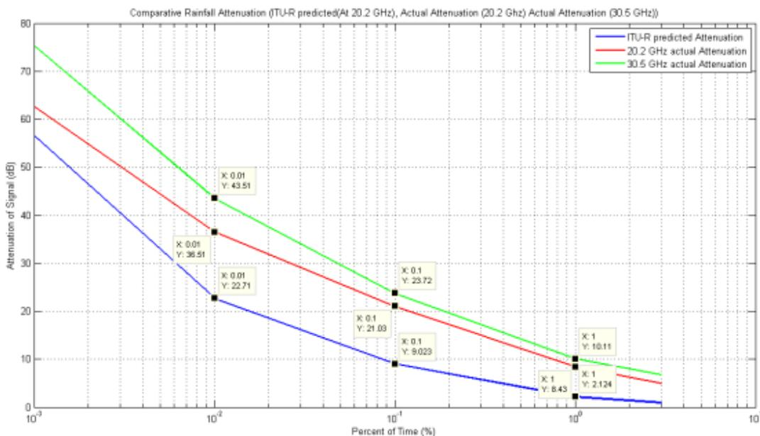
Fig. 3 — Comparative analysis of rainfall attenuation for Umiam, ITU-R predicted Attenuation vs. Actual attenuation (20.2 GHz and 30.5 GHz)
