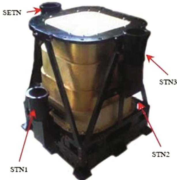
Fig. 14 — The schematic view of LEND instrument<sup>9</sup>.
