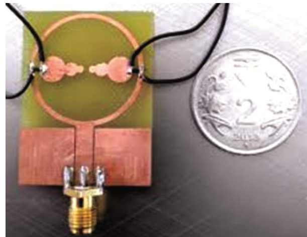
Fig. 9 — Prototype of proposed circular ring- shaped radiating patch antenna 17 .
