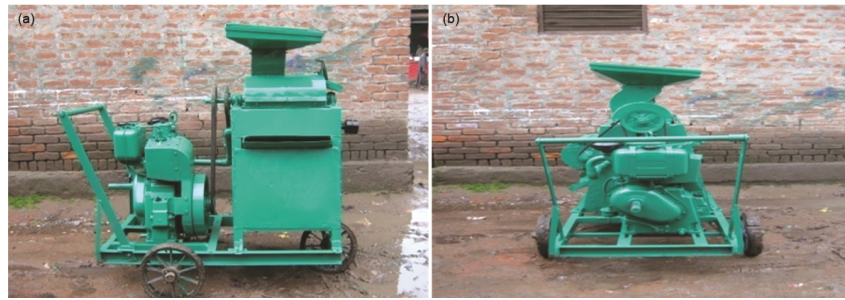
Fig. 3 — (a) Lateral view of the innovative Maize Sheller (b) Lateral (Motor) view of the innovation
