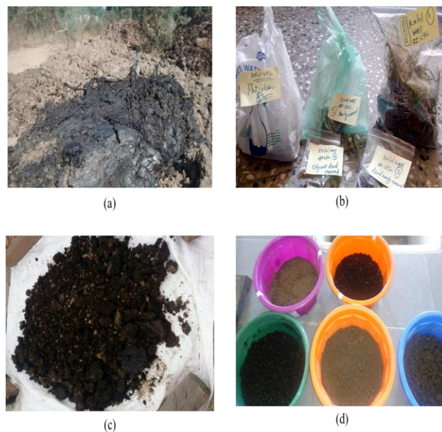
Figure 1: (a) Contaminated site at ONGC Kalol well no. 292; (b) Sample inoculates collected from five different zones of well no. 292, Kalol for preparation of inoculum; (c) Raw material provided from Kalol well no. 104 containing crude oil contaminated soil; (d) Experimental batch set-up for in-situ bioremediation.
