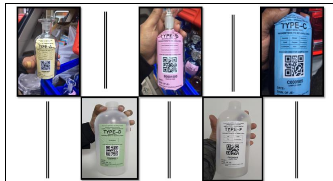
Figure 4: Various types of bottles required for the water sampling purpose
