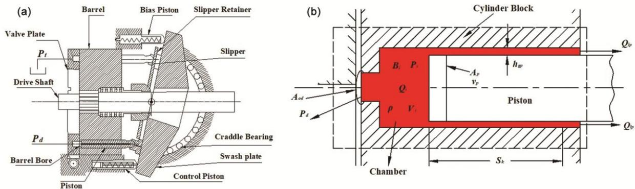
Fig. 1 — Schematic system diagram (a) Axial piston pump considered under study, (b) Control volume for the development of pressure in the piston chamber
