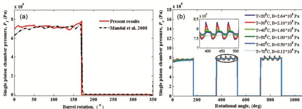
Fig. 2 — (a) Validation of single-piston chamber pressure and, (b) Effect of different temperature on single piston chamber pressure at a discharge pressure of 7.1MPa
