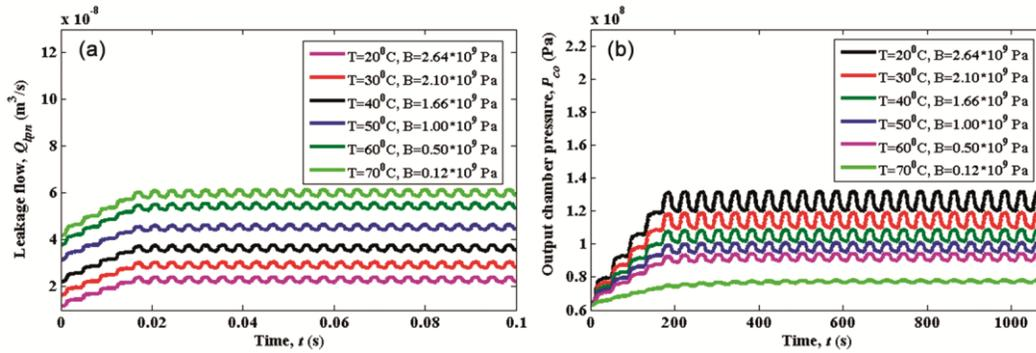
Fig. 3 — Effect of temperature on (a) Leakage flow, (b) Output piston chamber pressure
