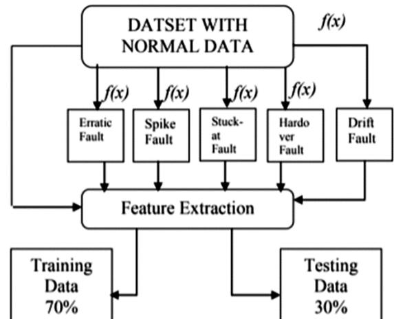
Fig. 3 — Dataset preparation procedure to train fault classifier
