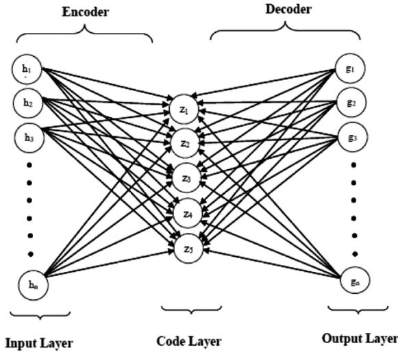
Fig. 4 — Architecture of fully connected Autoencoder network
