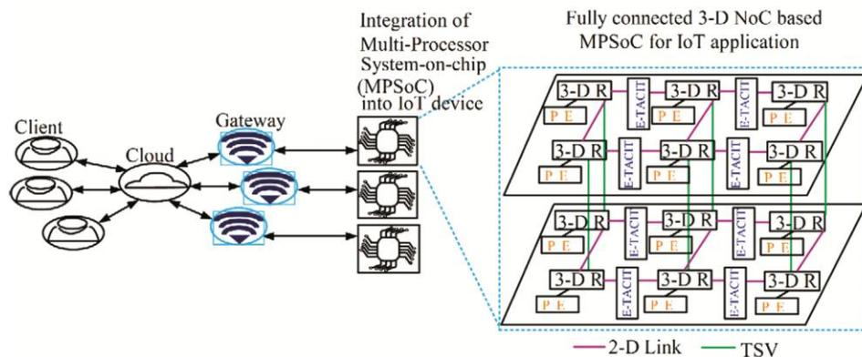
Fig. 2 — Symmetric 3-D NoC Architecture for IoT SoC Design
