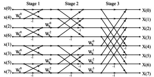
Fig. 4 — Signal Flow Graph for Radix-2,8-Point FFT
