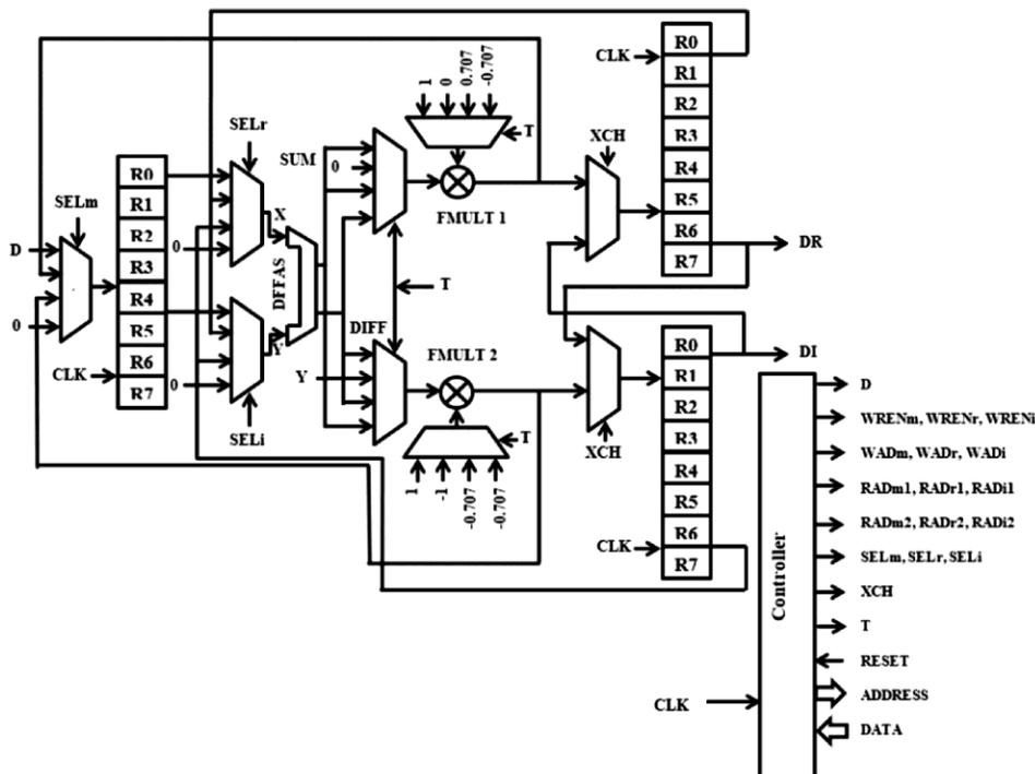
Fig.1 – Proposed FFT Architecture
