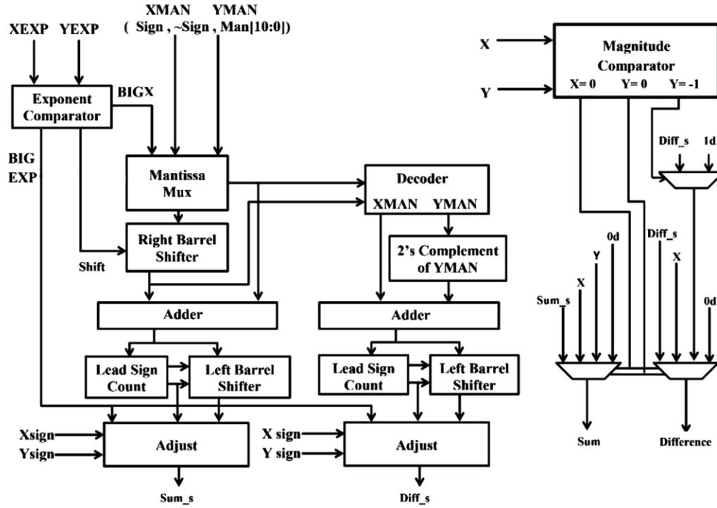
Fig. 2 — Dual Path Fused Floating Point Addition-Subtraction
