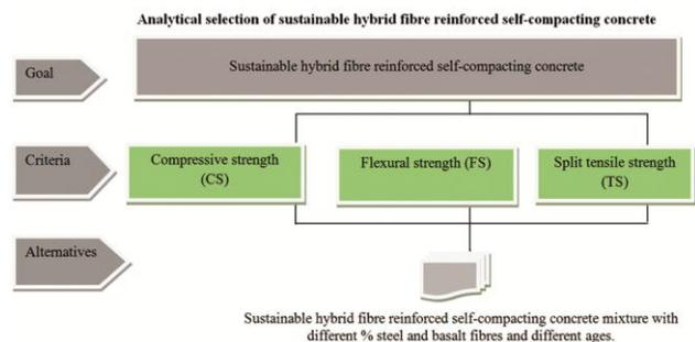
Fig. 1 — Schematic diagram for AHP analysis to select the sustainable hybrid fibre reinforced self-compacting concrete
