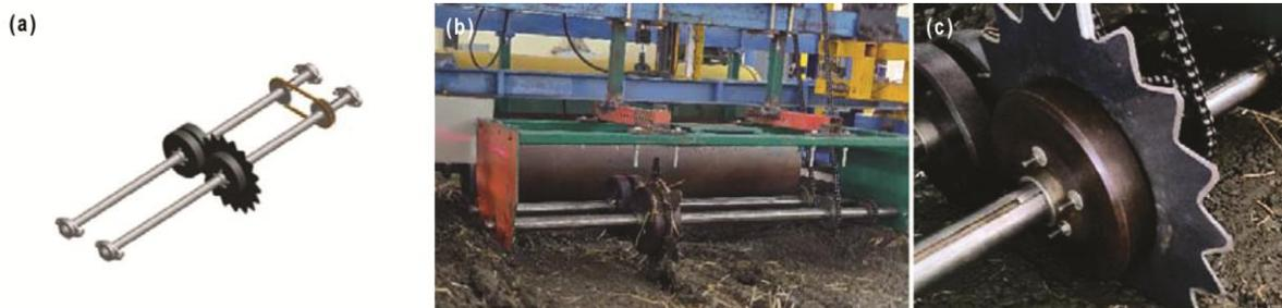
Fig. 2 — Disc coulters and press wheels mounted on the shafts of residue cutting system
