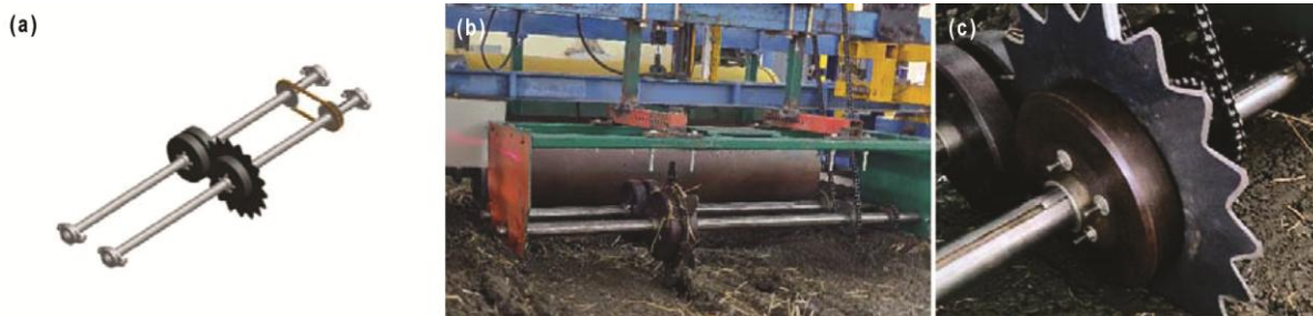
Fig. 2 — Disc coulters and press wheels mounted on the shafts of residue cutting system
