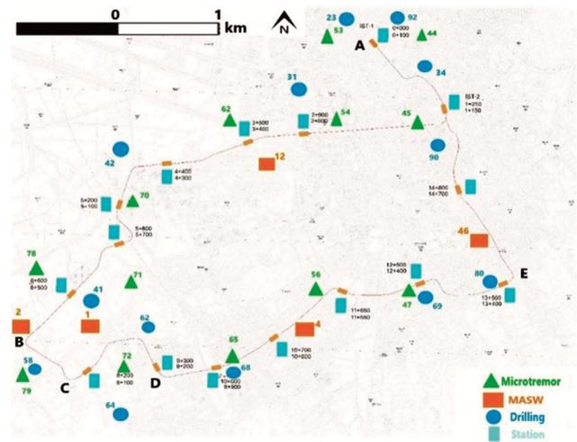
Fig. 4 — Locations of microtremor, borehole and MASW are located in areas close to the LRS route
