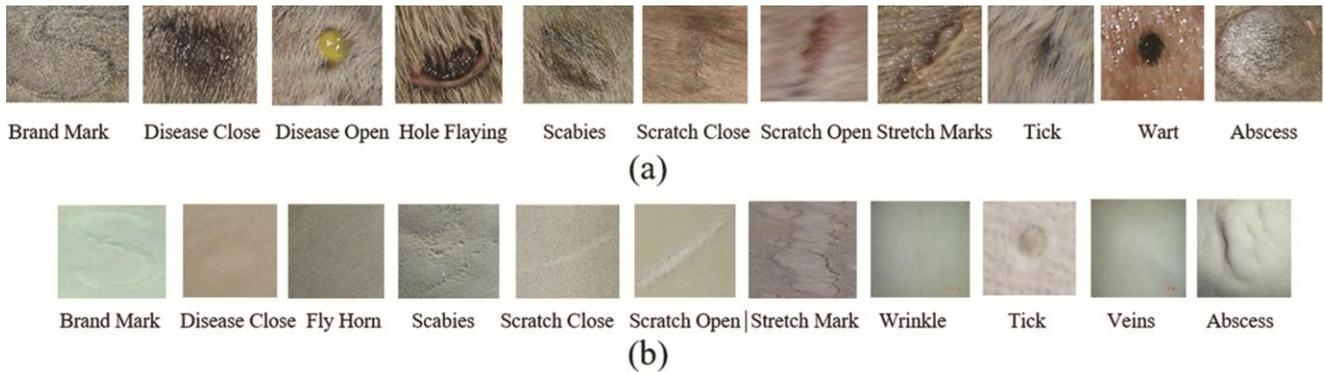
Fig. 1 — Samples of (a) Raw Hides and (b) Wet Blue Leather
