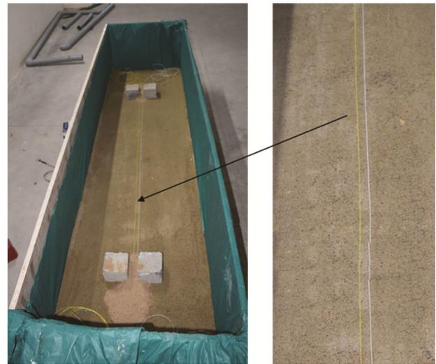
Fig. 6 — Distributed fiber optic sensor for leakage monitoring
