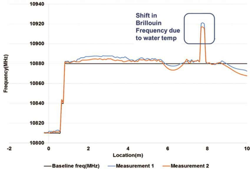
Fig. 4 — Brillouin frequency shift due to temperature variation
