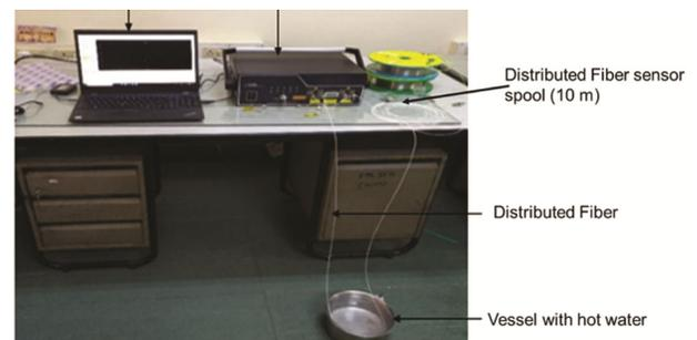
Fig. 3 — Temperature calibration of optical fiber
