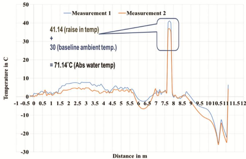
Fig. 5 — Temperature variation measured using Brillouin scattering
