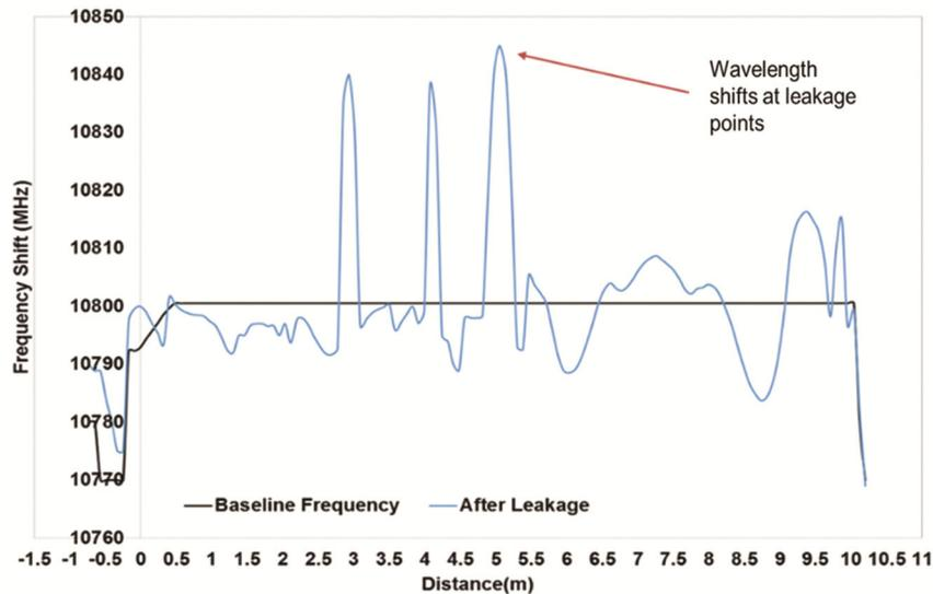
Fig. 8 — Brillouin frequency shift due to leakage in pipeline
