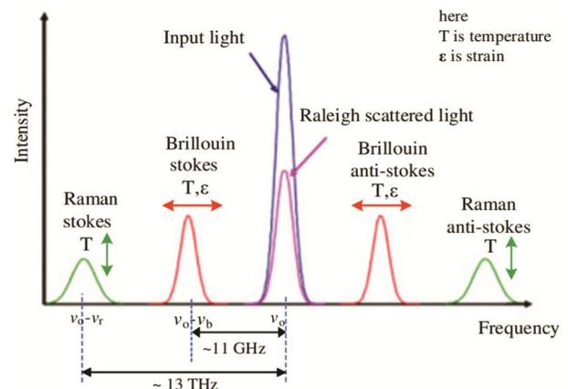
Fig. 1 — Scattering of light in an optical fiber<sup>35</sup>
