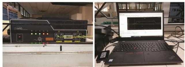
Fig. 7 — Data acquisition system in BOTDA mode
