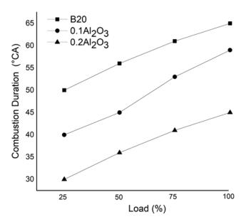
Fig. 5 — Variation of combustion duration with varying load
