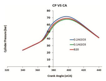
Fig. 3 — Variation of cylinder pressure with varying crank angle
