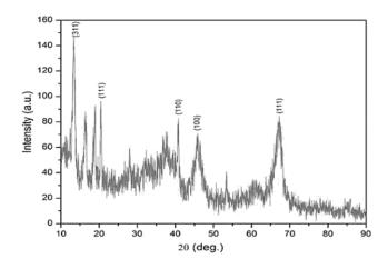
Fig. 1 — XRD patterns for Al<sub>2</sub>O<sub>3</sub> nanoparticle
