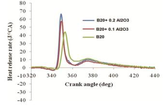
Fig. 2 — Variation in heat release rate with changing crank angle method based on LabVIEW is used to track the data in real time.<sup>5</sup>
