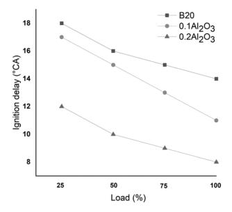
Fig. 4 — Variation of ignition delay with varying load
