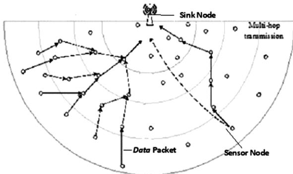
Fig. 4 — Route Setup for Non-Critical Data Transmission
