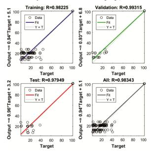
Fig. 12 — Comparison of the simulation results and predicted results derived from the ANN model for training, validation and testing, as well as in all three combined.
