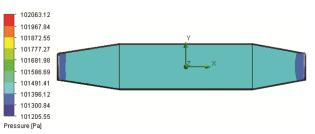
Fig. 6 — Pressure Values - Diffuser Length 140 mm (without distributor plate)
