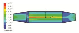
Fig. 9 — Velocity Values - Diffuser Length 140 mm (with distributor plate at 109 mm from leading edge)
