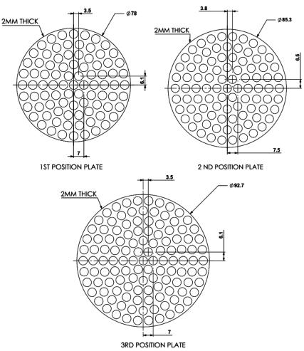
Fig.1 (b) — Distributor plates used in the catalytic converter
