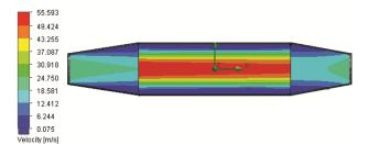
Fig. 8 — Velocity Values - Diffuser Length 140 mm (without distributor plate)
