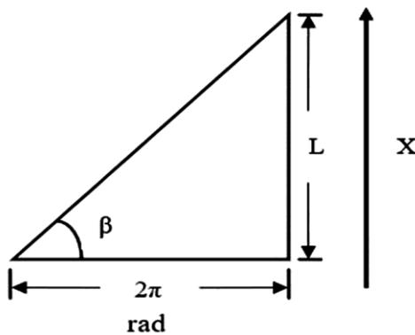
Fig. 3 — Relation between angular and linear displacement
