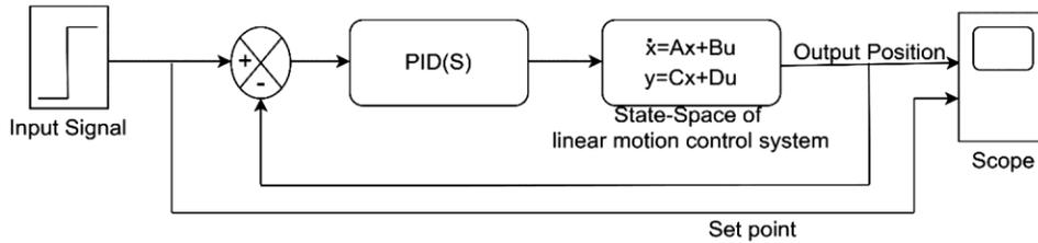
Fig. 5 — Simulink model of PID controller
