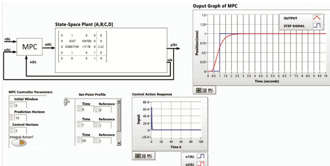
Fig. 10 — Front panel of MPC in Lab VIEW
