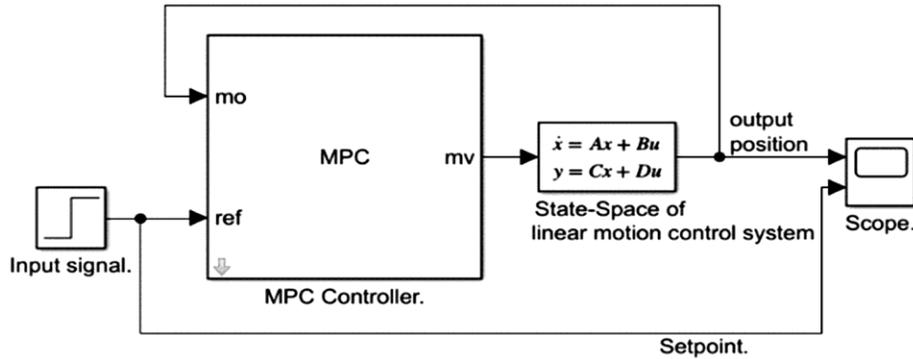
Fig. 8 — Simulink model of MPC controller
