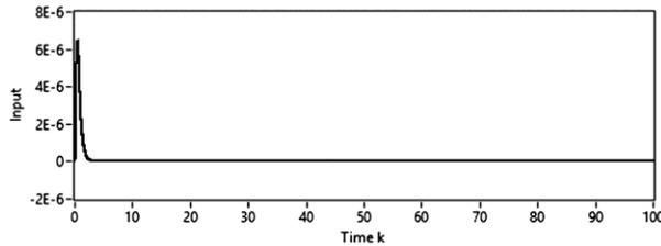
Fig. 16 — Control action response of MPC in Lab VIEW
