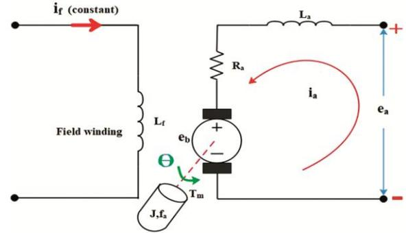
Fig. 1 — Electrical circuit for DC servo motor
