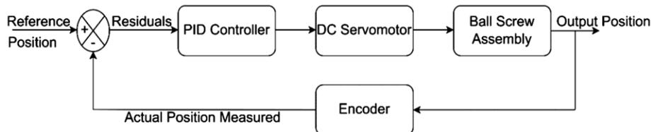
Fig. 4 — PID controller block diagram
