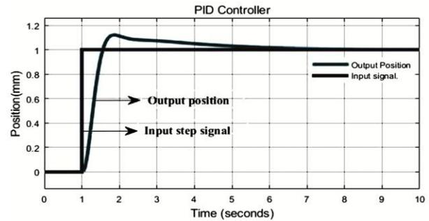
Fig. 11 — Step response of PID controller
