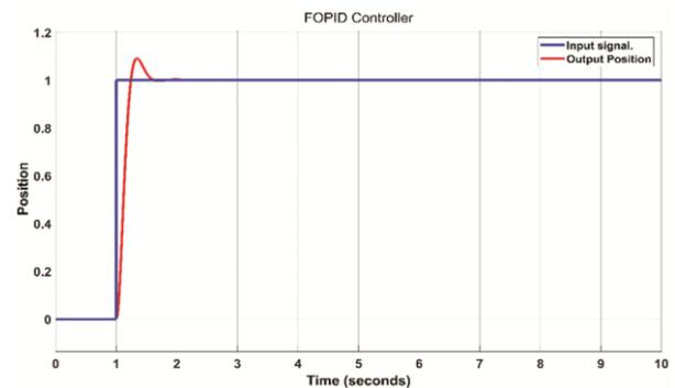
Fig. 12 — Step response of FOPID controller
