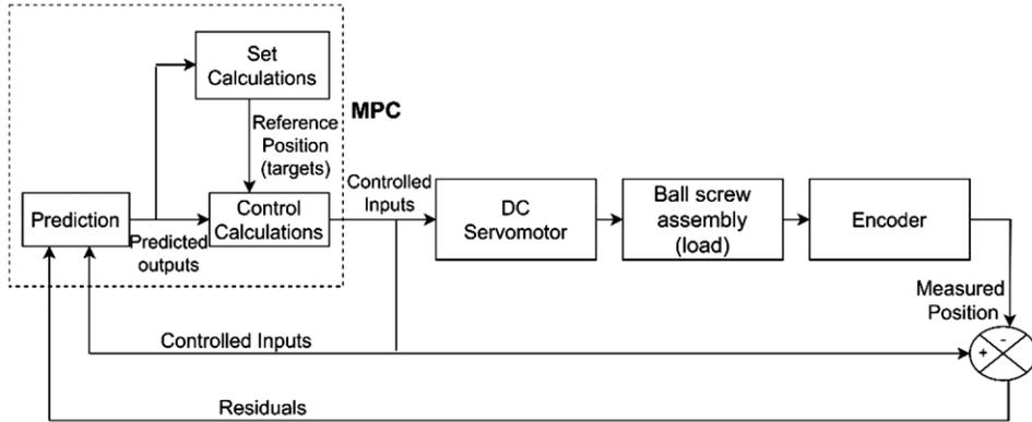
Fig. 6 — Block diagram of MPC
