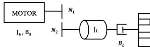
Fig. 2 — DC servo motor with rotational load
