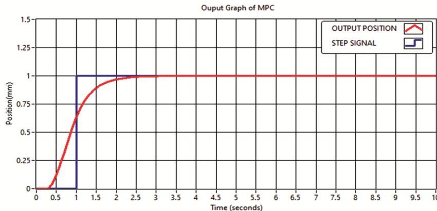
Fig. 15 —Step response of MPC in Lab VIEW
