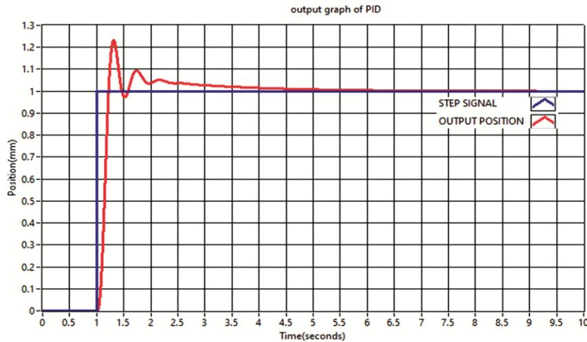
Fig. 14 —Step response of PID in Lab VIEW
