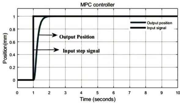
Fig. 13 — Step response of MPC controller
