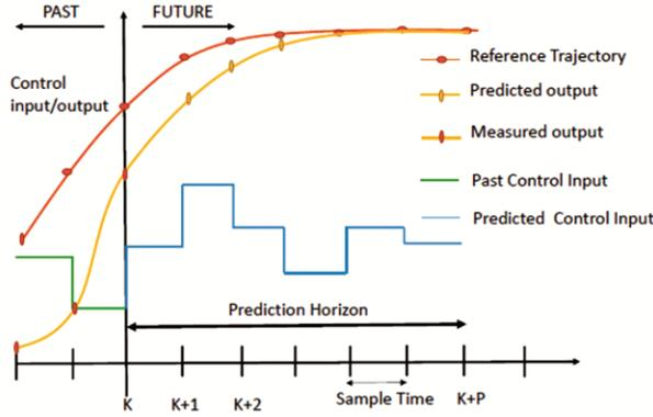
Fig. 7 — Graphical representation of MPC
