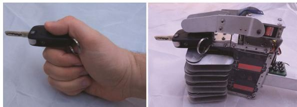
Fig. 12 — Comparison of the lateral pinch
