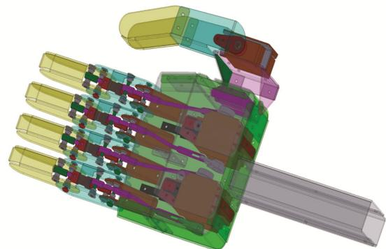
Fig. 4 — The angle view of the proposed robotic hand 3D model designed in Solid Works
