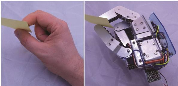
Fig. 11 — Comparison of the tip pinch
