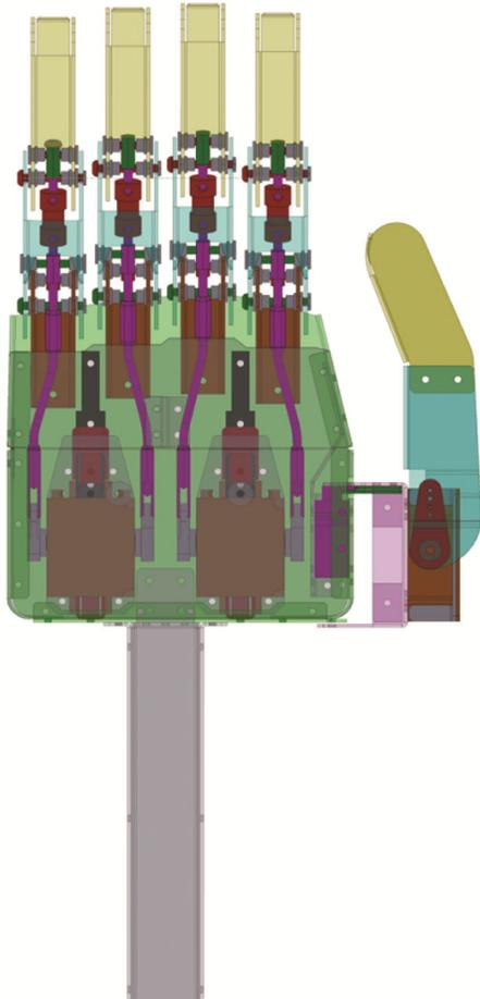
Fig. 3 — The top view of the proposed robotic hand 3D model designed in Solid Works
