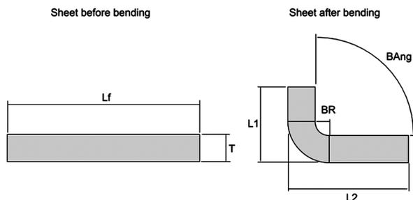
Fig. 5 — Parameters of aluminum sheet for K-Factor calculation
