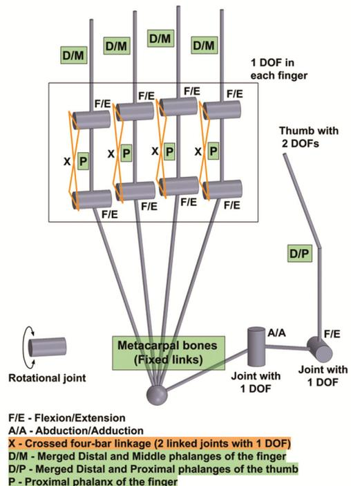
Fig. 2 — Kinematic model of the designed robotic hand; the colors in legend correspond to the parts
