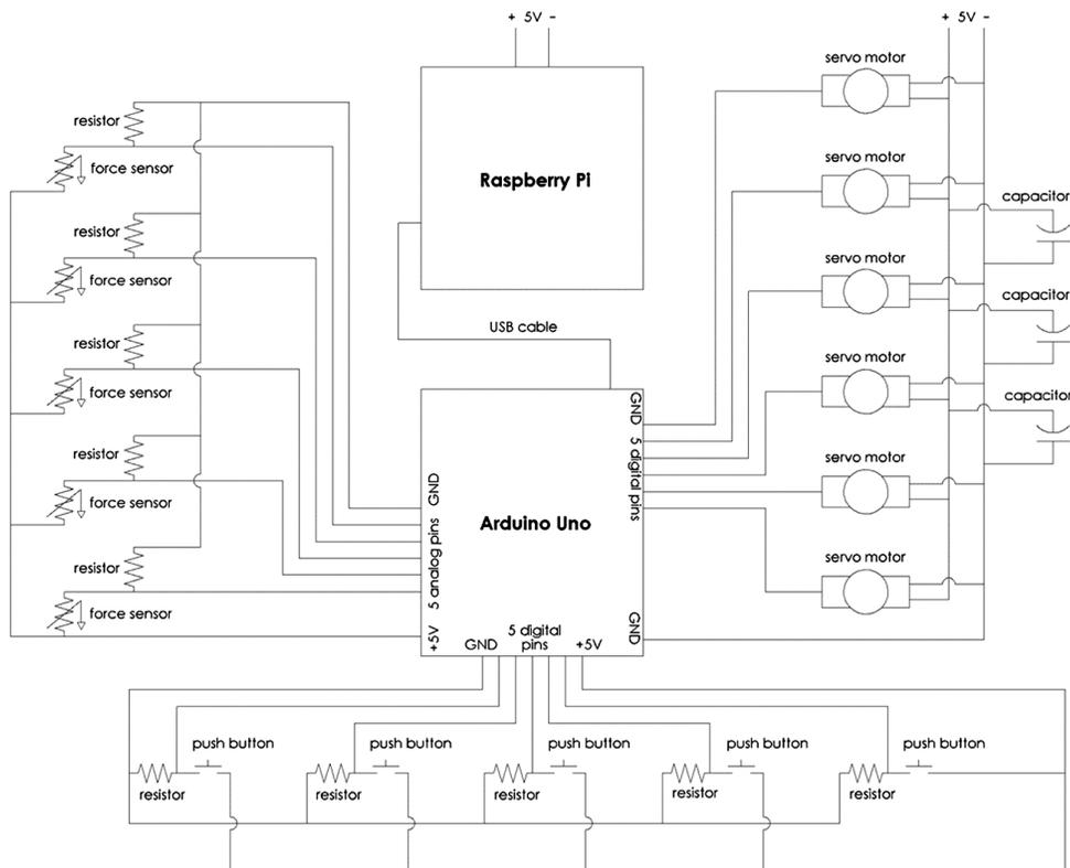
Fig. 8 — Electronic circuit of the robotic hand
