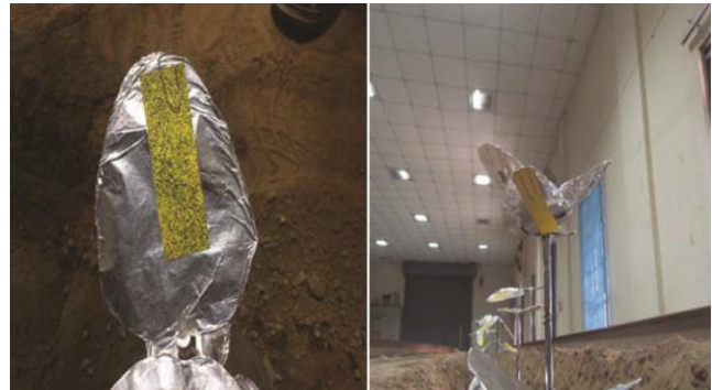
Fig. 3 — Adaxial and abaxial deposition of spray liquid on water sensitive paper attached to artificial cabbage leaves
