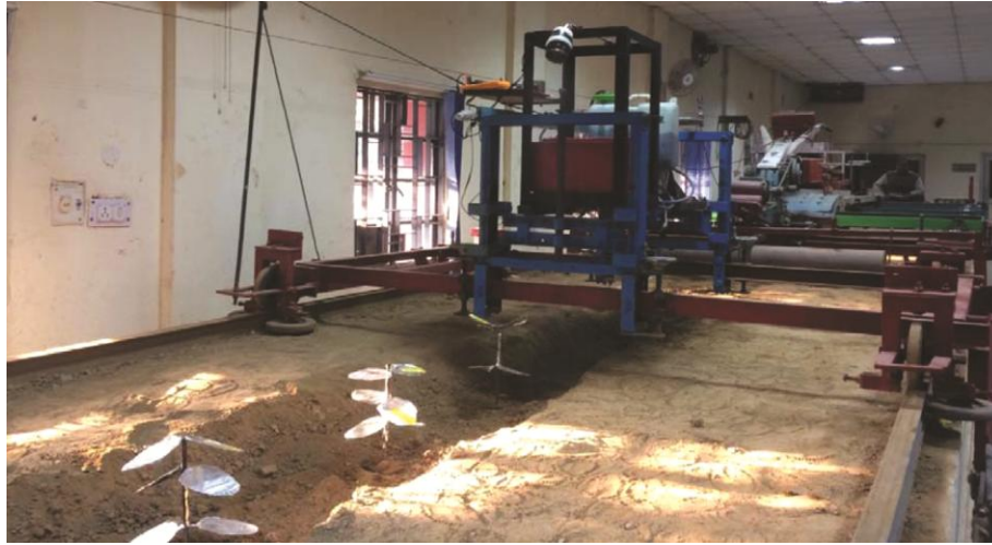
Fig. 2 — Experimental setup to study effect of operational parameters on deposition efficiency of spray droplets on artificial leaves
