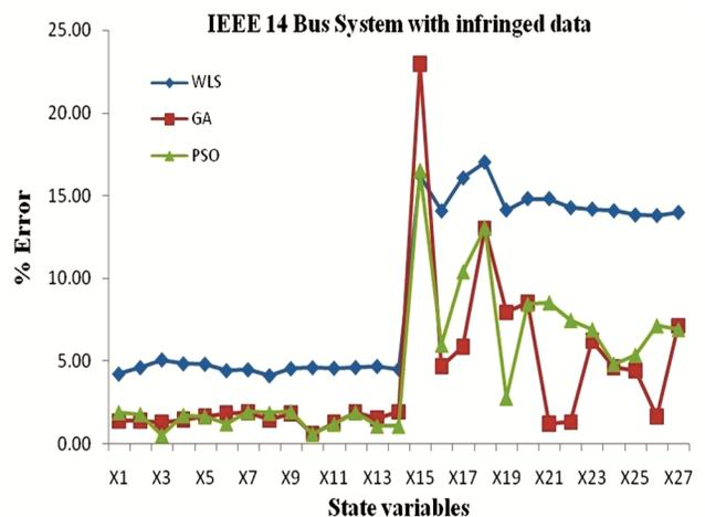
Fig. 17 — Variation in % error with infringed data – IEEE 14 Bus
