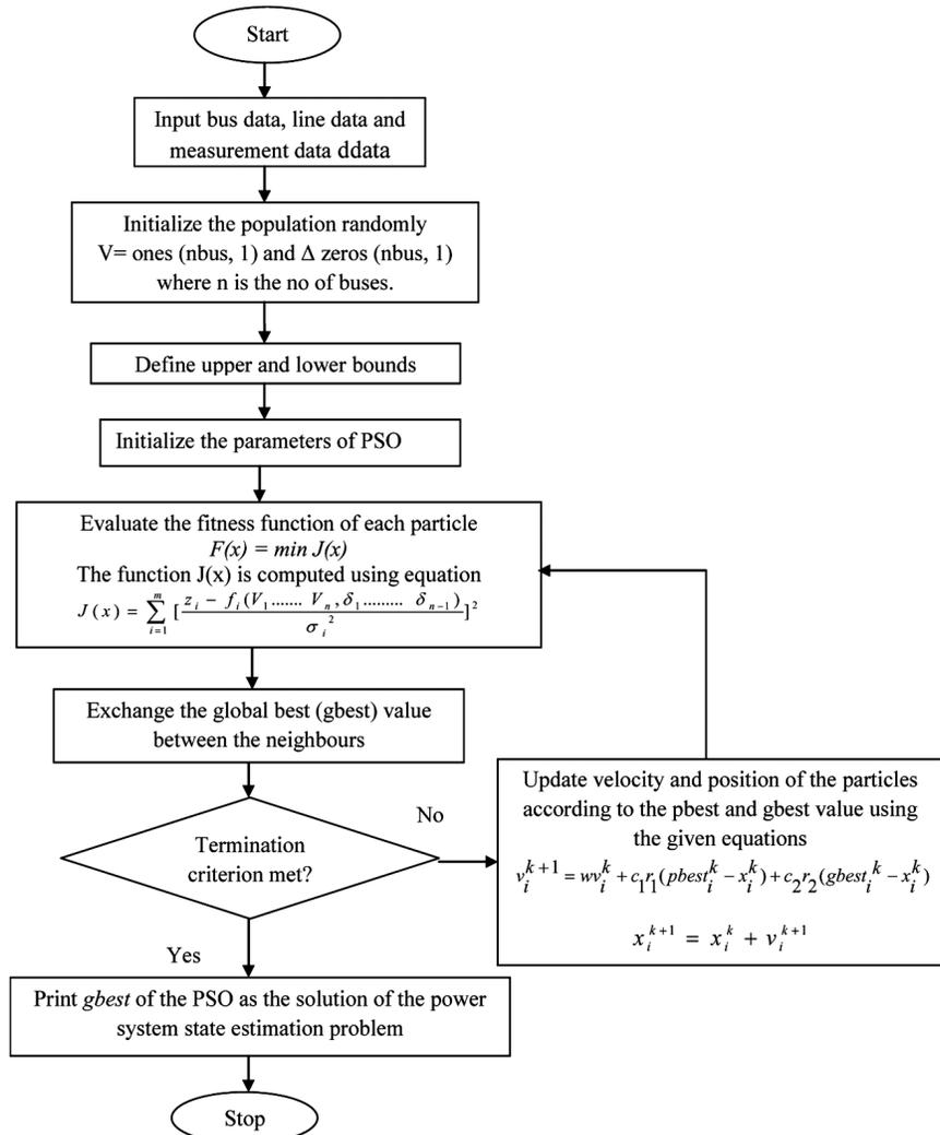
Fig. 3 — Process flow chart of implementation of PSO for state estimation
