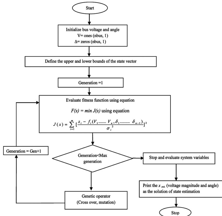
Fig. 2 — Process flow chart of implementation of GA for state estimation
