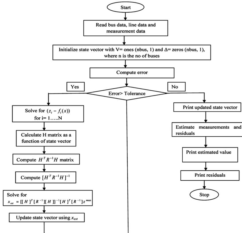
Fig. 1 — Process flow chart of implementation WLS for state estimation
