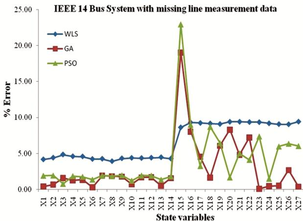
Fig. 15 — Variation in % error with missing data – IEEE 14 Bus
