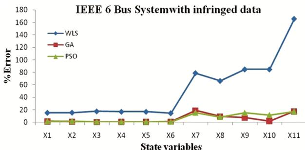
Fig. 11 — Variation in % error with infringed data – IEEE 6 Bus
