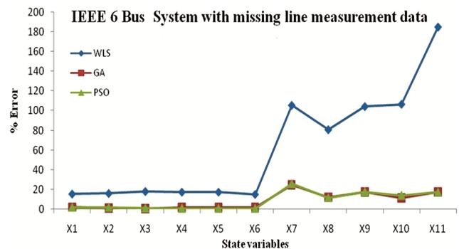
Fig. 9 — Variation in % error with missing data – IEEE 6 Bus
