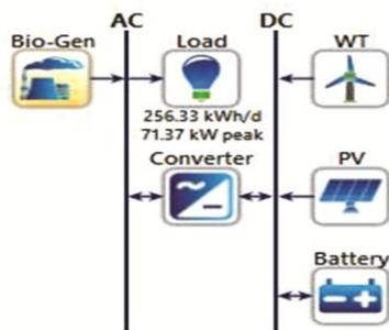
Fig. 1 — Hybrid system model designed in Homer Pro
