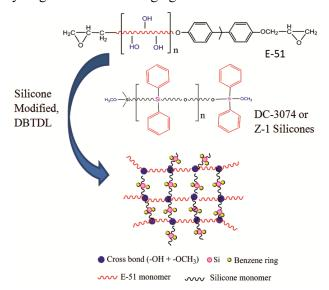
Fig. 1 — Scheme for silicone modified epoxy resin
