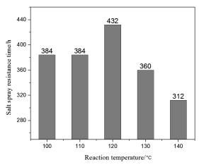
Fig. 7 — Effect of reaction temperature on the salt spray resistance time of coatings
