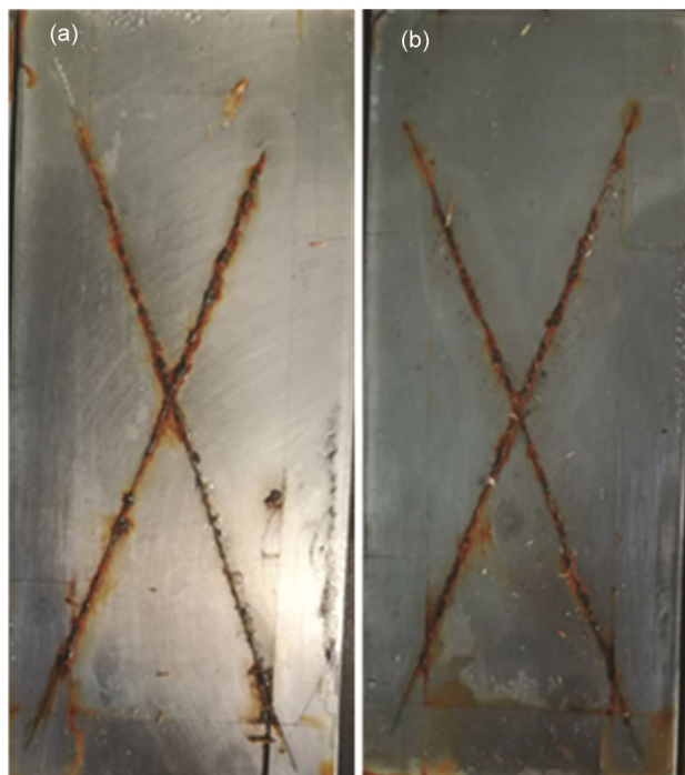
Fig. 5 — Comparison of salt spray resistance of different silicone modified epoxy resins: (a) DC-3074 modified epoxy resin, (b) Z-1 modified epoxy resin
